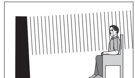
**Figure 11–12.** A controlled 30 degree cylindrical wave-front, a MartinLogan exclusive, offers optimal sound distribution with minimal room interaction. The result is solid imaging with a wide listening area.
