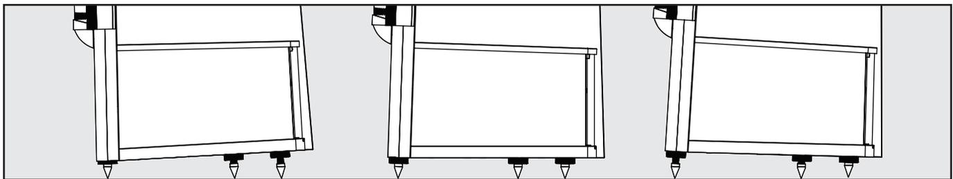
Figure 6. Adjust rake of the CLX by varying the height of the jam nut, and/or by removing the jam nut.
