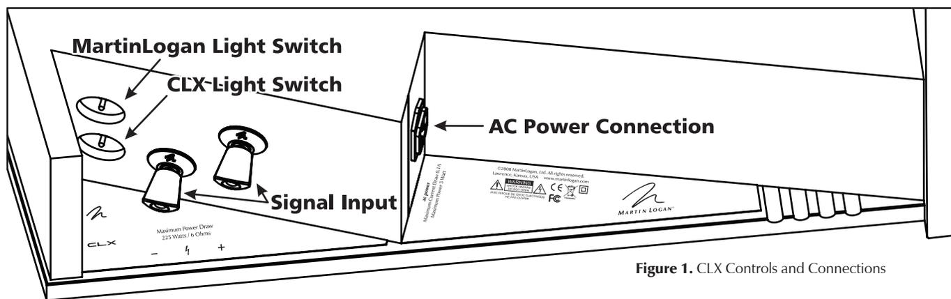
Figure 1. CLX Controls and Connections
