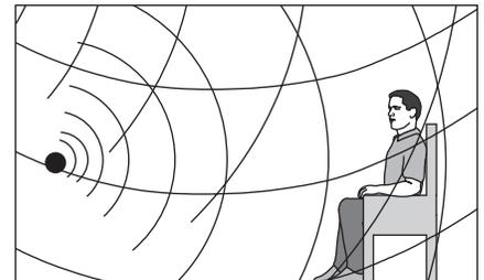
**Figure 9–10.** Even though they suffer from “venetian blind” effect, angled multiple panel speakers can deliver good imaging, but only to specific spots in the listening area.
