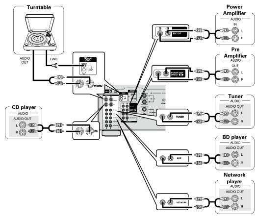
If humming or other noise is generated when the ground wire is connected, disconnect it.
