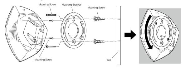
Mount the Extend on the mounting bracket by rotating the unit clockwise about 90 degrees to secure it in place.
