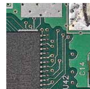
Digital Signal Processing is built onto a replaceable module.
