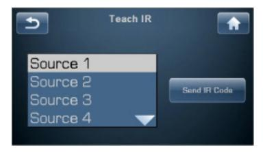
The Teach IR page displays a scrolling list of all the available IR codes in the CP-800. Simply scroll to the command you want your macro-capable remote to learn and touch the **Send IR Code** button. The CP-800 continuously sends that command code via the front panel - as long as the button is pressed – until your third-party remote control has learned it.
