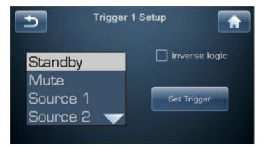
The triggers can be associated with the Standby mode, a specific source or a configuration. To use the Inverse Logic option, simply check the Inverse Logic box on the Trigger Setup page.
