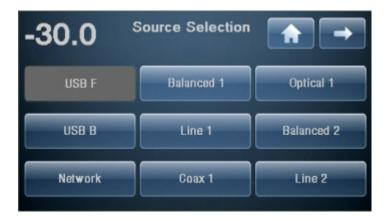
Touch any **source** button on the touchscreen to select it as the current source. The selected source button is shaded. If the source you want to choose is not on this screen (and you have more than nine source buttons enabled), press the button for the next page of sources. Or, press the button to return to the previous page.
