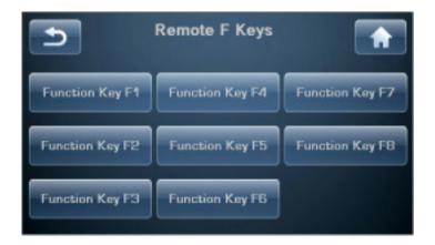
The remote control **F1** to **F8** buttons correspond to the Function Keys displayed on the touchscreen. Select the **Function Key** that you would like to assign, then scroll through the list and choose the specific function you want that **Fkey** to perform.
