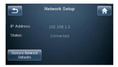
The CP-800 includes a built-in web interface that can be used to configure the system name, Network settings or update the CP-800 software. To access the interface, type the IP address displayed on the Network Setup page in the URL line of your browser (e.g. 192.168.1.0) and hit return. Alternately if you are using Safari on the Mac, you can "Show All Bookmarks" (See: Bookmarks menu) and click on Bonjour and double click on your CP-800 device listed in the Webpage's folder.
